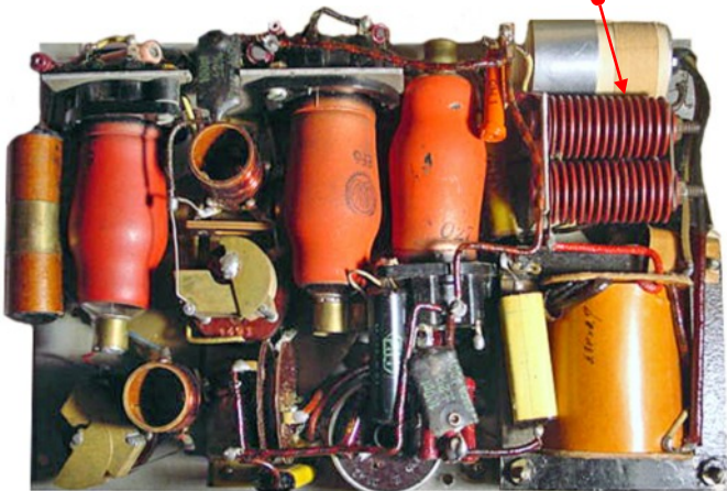
Internal view of OSB type II s/n 905 (using a 6H6 rectifier valve above) and that of s/n 952 (below). Note a selenium rectifier in s/n 952.
